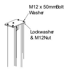
**STEP 6**: Position the columns facing each other **138-1/2**" outside base plates. Square the columns by measuring diagonally from corner points on base plates (within 1/4"). See plan and elevation drawings on page 4 for detailed drawing.
