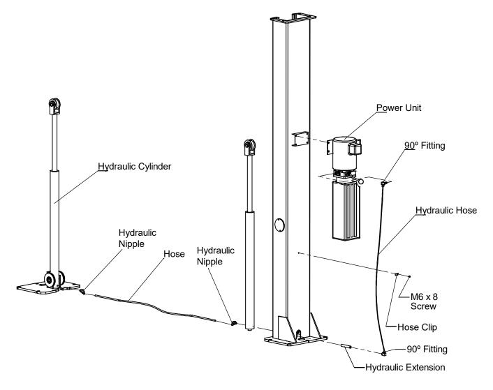
STEP 13 Mount the Power Unit on lift as shown.
