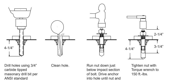
**STEP 8:** Using a level, check column for side-to-side plumb and front-to-back plumb. If needed, use horseshoe shims provided by placing shims underneath the base plate and around the anchor bolt. This will prevent bending the column bottom plates (Shim thickness should not exceed 1/2"). Tighten 3/4" anchor bolts to **150 ft-lbs.** of torque.
